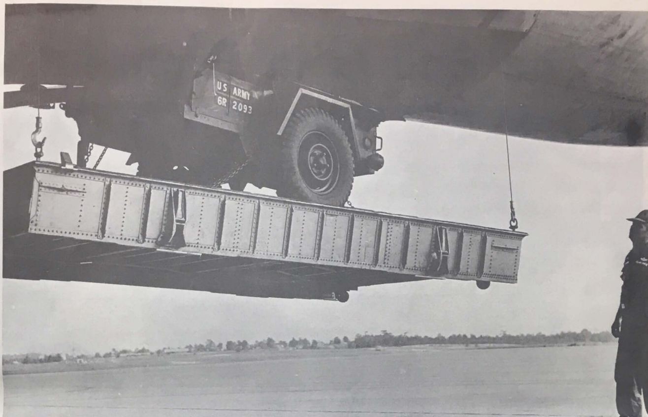
A three-quarter ton trailer disappears into the belly of a C-124.
